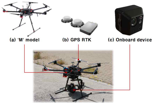
Figure 1. Configuration of prototype industrial drone
