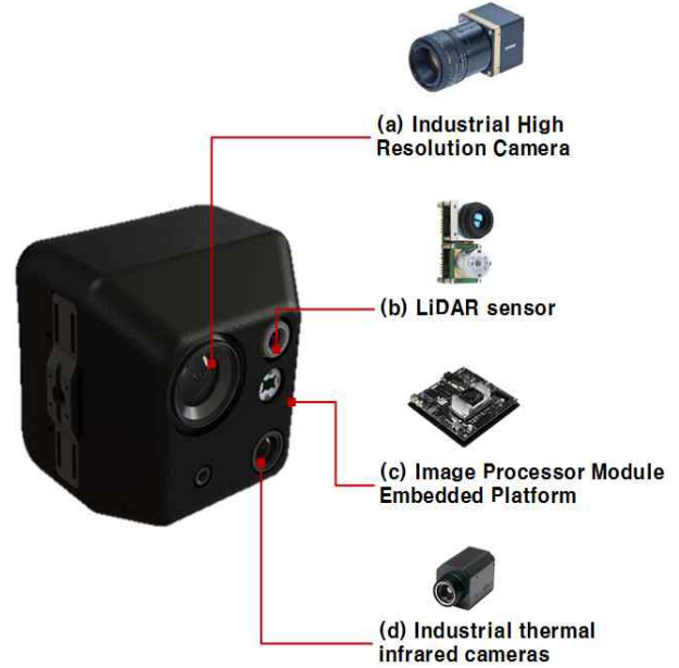
Figure 2. Configuration of onboard devices
