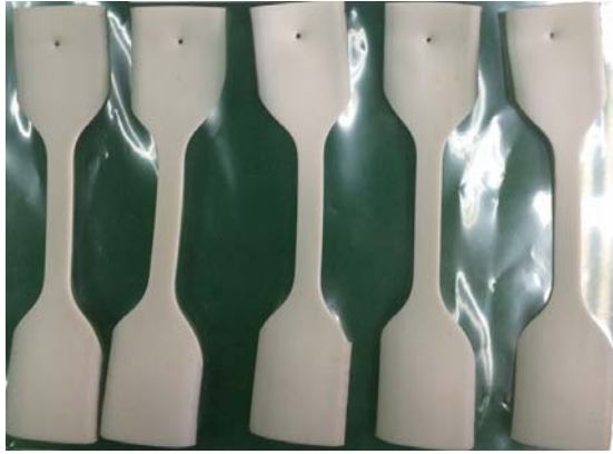
Figure 1. Specimen of cable jackets for nuclear power plants
