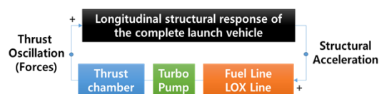
Fig. 1 Closed-loop system of the pogo phenomenon.
