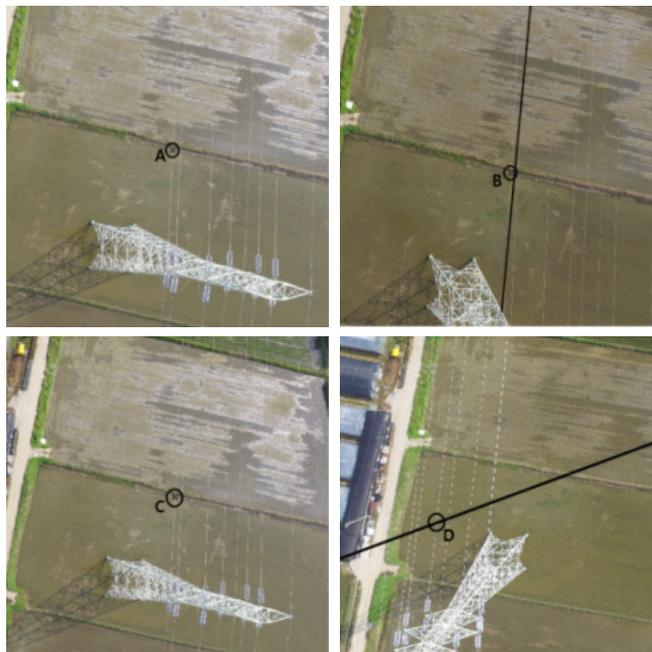
Fig. 5. Use of epipolar lines for 3D powerline mapping
