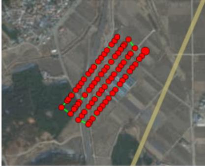
Fig. 3. Image acquisition grid (4 strips and 75 photos)
