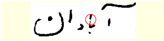
Fig. 3. Example of word-break as a result of binarization.
