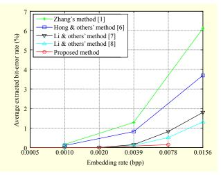
Fig. 7. Average extracted BER comparison.
