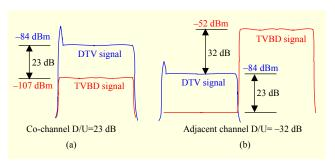
Fig. 4. (a) D/U ratio at grade B contour to protect DTV service from co-channel TVBD interference and (b) D/U ratio at grade B contour to protect DTV service from adjacentchannel TVBD interference.
