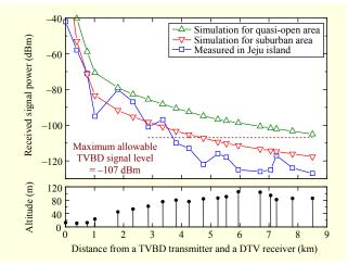
Fig. 12. Received interference signal power at ATSC DTV receiver with antenna height of 10 m; interference signal is transmitted from signal generator with transmitting antenna height of 10 m, which is located at distance ranging from 10 m to 8.5 km from DTV receiver.
