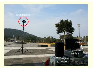
Fig. 6. Interference measurements from TVBD into WM receiver in front of Jeju Art Center in Korea.
