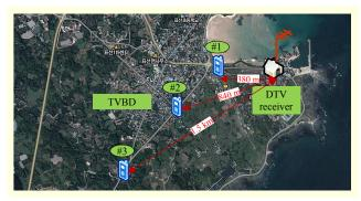
Fig. 11. Field test for required separation distance verification of 100 mW portable TVBDs in rural area near beach.
