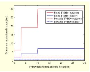
Fig. 7. Co-channel separation distance of TVBDs from noiselimited contour for both indoor and outdoor WM service.
