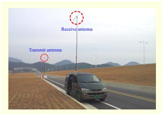
Fig. 2. Field strength measurement van.
