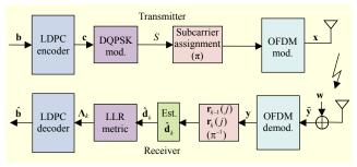
Fig. 1. System model of differential encoded blind transceiver design with LDPC code under SISO-OFDM signaling.
