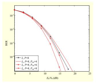
Fig. 8. BER performance of TSFE method with channel-order mismatch and optimal interleaving using 512 OFDM subcarriers and Doppler frequency of 0 Hz.
