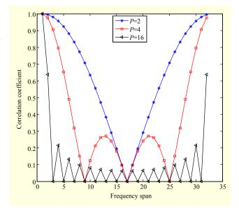
Fig. 2. Auto-correlation of OFDM subcarriers for P = 2, 4, and 16 (for 32 subcarriers).
