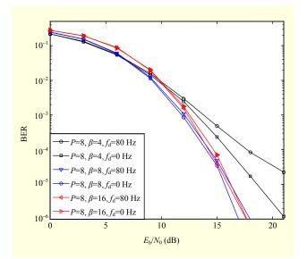
Fig. 4. Effect of spreading factor  $\beta$  on diversity: P = 4, with 1,240 OFDM subcarriers and Doppler shifts of  $f_d = 0$  Hz and 80 Hz.
