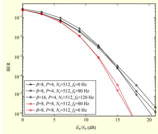
Fig. 5. Impact of number of paths *P* of SISO-OFDM system on BER performance of TSFE method.
