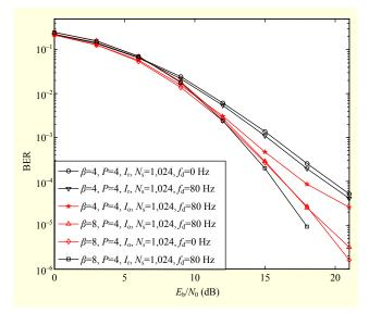
Fig. 3. BER performance of optimal and random interleaving for 1,024 subcarriers: P = 4; spreading factors of  $\beta = 4$  and  $\beta = 8$  at Doppler frequencies of 0 Hz and 80 Hz.
