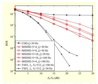
Fig. 6. BER performance of TSFE method vs. MSDSD method [17] using P = 4 and  $\beta = 4$ .
