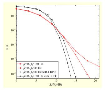
Fig. 7. BER performance of TSFE method with LDPC (648, 324) and without LDPC for different spreading factors.
