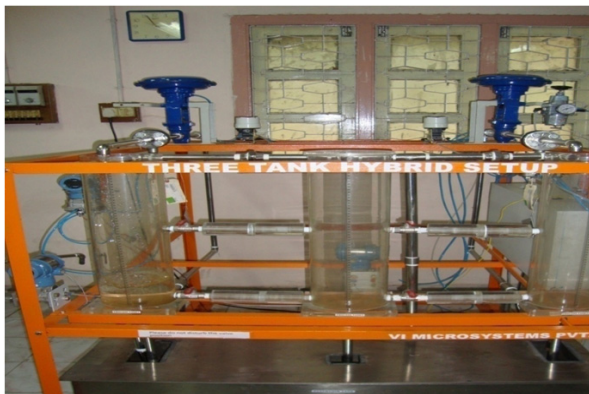
Fig. 4 Experimental set up of hybrid three-tank system
