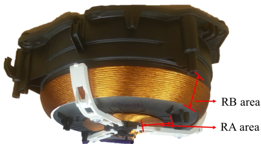
Fig. 6. Primary winding and thermal insulator structure
