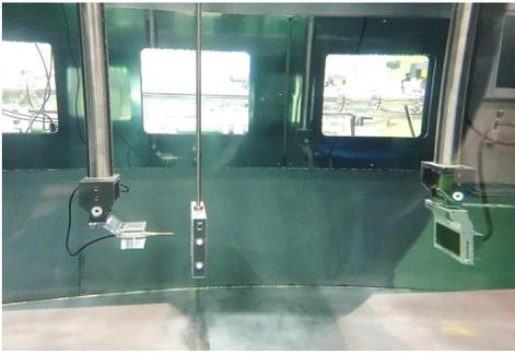
Fig. 7 Immersion test setup to measure the longitudinal wave speed of the polymethylpentene
