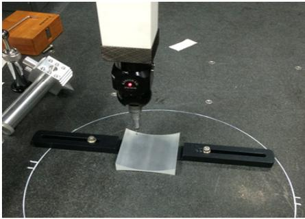
Fig. 11 Setup to measure the lens shape
