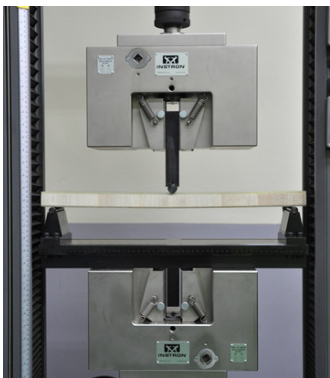
Fig. 4 Three points bending test
