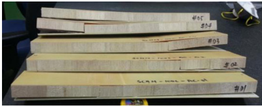
Fig. 10 Fracture of sandwich panel
