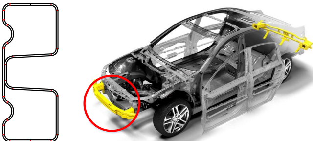
Fig. 1 Cross section and shape of bumper beam
