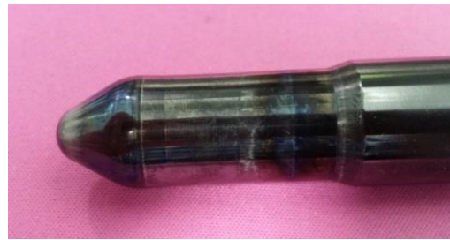
Fig. 8 Outlook of the primary punch after several ten thousands of forging times
