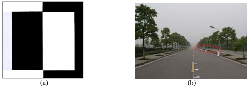
Fig. 13. Reference targets and their positions. (a) Ideal black-and-white target. (b) Target positions.
