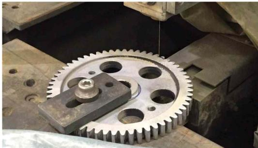
Fig. 6. Artificial production of defective specimens using spur gear cutting wire.
