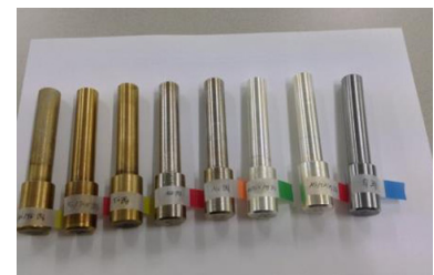
(c) Coating bolts
