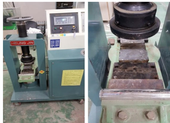
Fig. 7. Photos of flexural strength test
