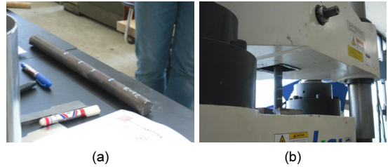
Fig. 5. Specimen preparation and tensile strength test : (a) specimen for tensile strength test, (b) tensile strength test
