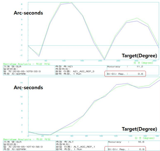
Fig. 20. Analysis of repeated point accuracy (Up : Azimuth / Down : Altitude)
