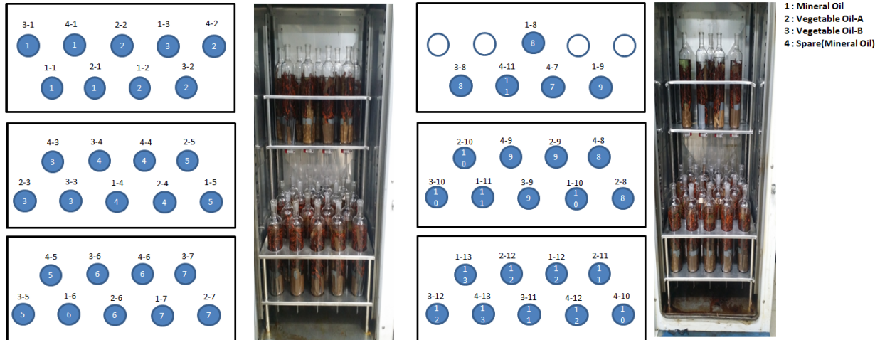
Fig. 1. Accelerated Aging System(Test cell & Tray)
