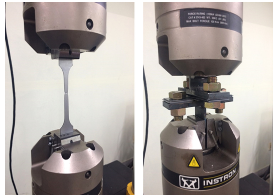
Fig. 6 Tensile test equipment and specimen setting
