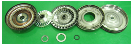
Fig. 2 Components of torque converter
