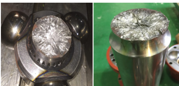
Fig. 14 Fracture surfaces after torsional fatigue test
