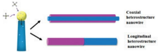
[Fig. 2] Heterostructure nanowires
