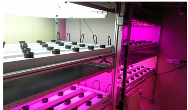
Fig. 1. Nutrient film technique (NFT) systems equipped with 3 types of combined LEDs and control (fluorescent lamps) in a closed-type plant production system used in this study.
