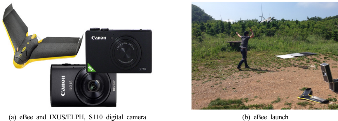
Fig. 2. UAV system and taking off for a mission.
