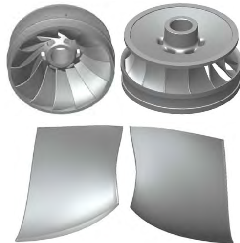
Figure 3: 3D modeling of the Francis hydro turbine model runner and blade shapes
