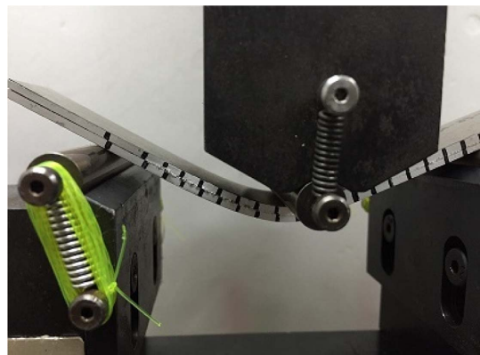
Fig. 6. Fracture during ENF test
