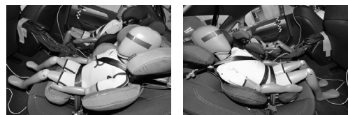
Fig. 4 Q6 (left) & Q10 (right) setting on rear seat in vehicle
