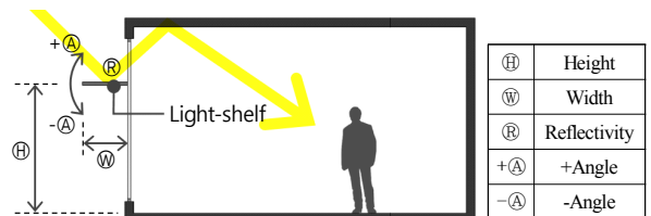
Fig. 2. Concept and variable of light-shelf
