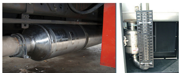
Figure 6. Explosion proof certified samples of diesel engine's exhaust spark arresters.
