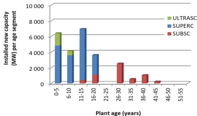
Figure 1. Type, operation period, electricity generation capacity of Korean coal-fueled electricity power plant
