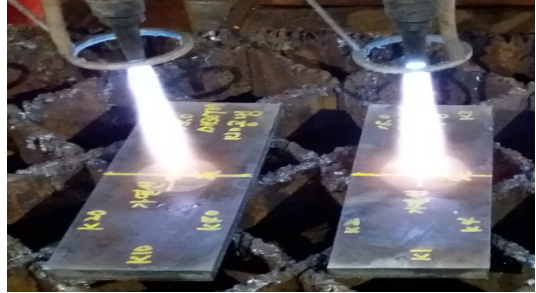
Fig. 3 Photo of line heating process by heating torch
