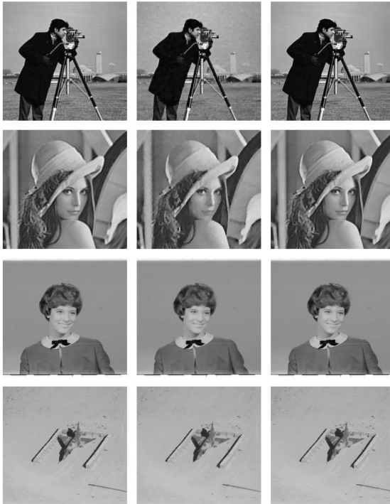
Fig. 3. Reconstructed images using N measurements; DCT coefficients only, DCT coefficients with TV recovery, and DCT and Noiselet coefficients with TV recovery from the left
