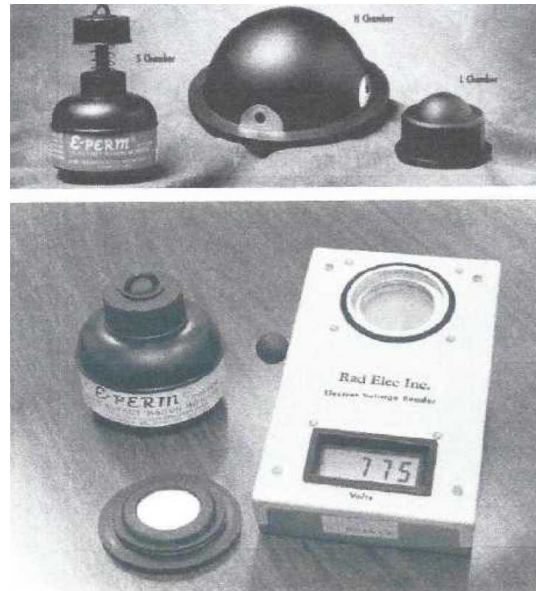
Fig. 1. E-PERM, Electret voltage detector and installation
