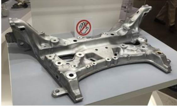
Fig. 10 Aluminum sub-frame by honda
