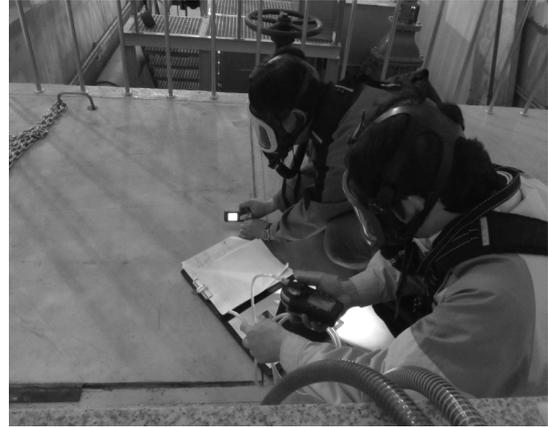
[Figure 2] Measurement of Gas Concentration
