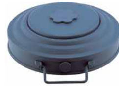
Fig. 4. Mock-up targets for the mine detecting test.
