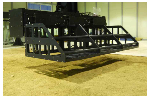
Fig. 5. MD performance test using the electrical controlled 3-axis scanner.
