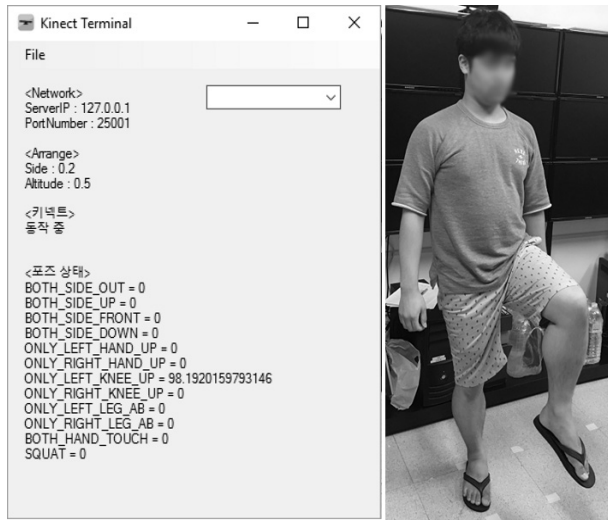
Fig. 6. Snapshot of Kinect-based Pose Recognition Model Experiment: C# Kinect Terminal (Left), LEFT_KNEE_UP Pose (Right)
