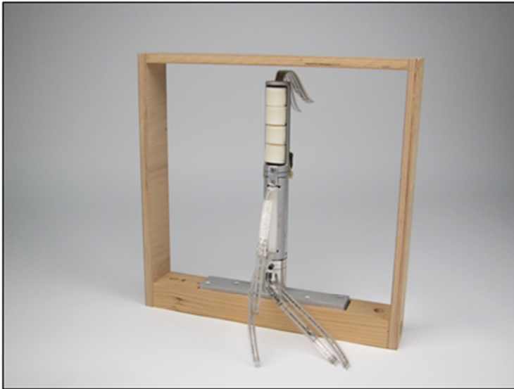
Figure 1. A custom-made equipment used for output (pushing, pulling, and twisting) and grip force measurement
