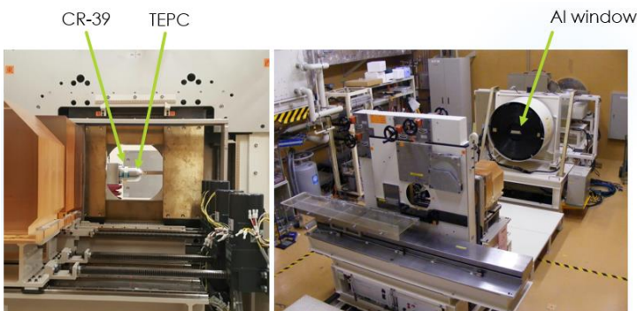
Fig. 1 Experimental setup of CR-39 in Bio. Laboratory of HIMAC
