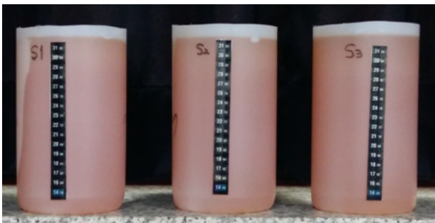
Fig. 1 TM phantom of cylinder type(a: PE phantom, b: CPP phantom, c: Talc phantom)
