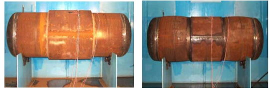
Fig. 8. Hydraulic test result after Type A(right side) and Type B(left side) sleeve repair[15].
