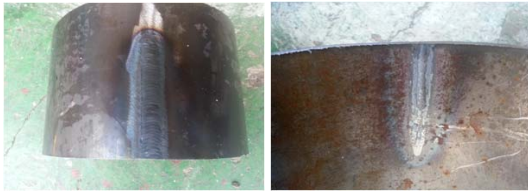
Fig. 7. An example repair with deposited welding metal.
