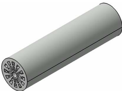
(b) Hollow shaft with a column
