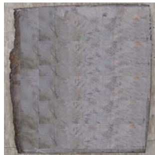
Fig. 4 Gr.91 steel plates sampled from a USC plant
