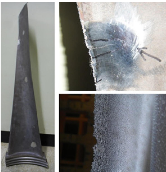
Fig. 4 Crack position on the last stage blade [2]
