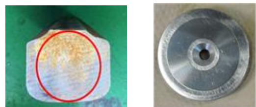
(a) Rail head part (b) Test specimen
