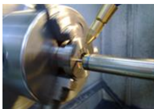
(b) UNSM device working on the specimen
