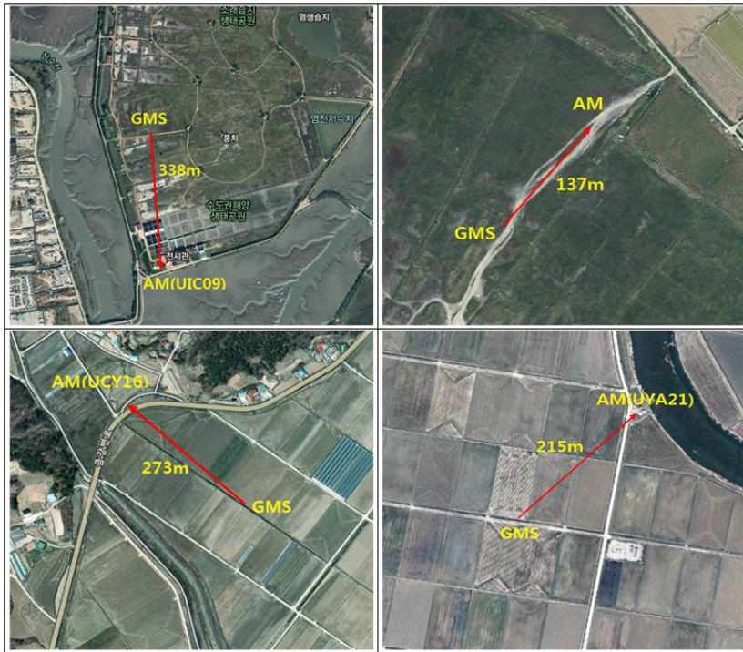
Figure 2. Overview of the geomagnetic absolute measurement stations near unified control points (GMS : Geomagnetic station, AM : Azimuth mark)
