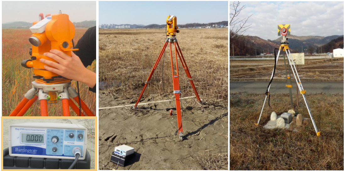
Figure 3. The declination-inclination magnetometer(Mag-01H, 0.1nT) consists of a single-axis fluxgate sensor(Mag type “A” Probe) mounted on a nonmagnetic theodolite(Zeiss 020B)
