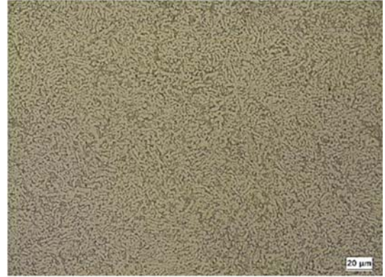
Fig. 1. Optical micrograph of the as-received Ti-6Al-4V ( \times 500 ).
